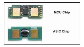
**IMPORTANT NOTE!!** If you even see a chip with a big black dot (it seems to be an ASIC one), the chip could be an MCU solution with just a plastic coverage.
